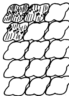
Figure 4. Diagram of the second type Nesbitt envelope, showing how rearranging the watermark emblems permitted rearranging the knives to produce three more envelopes from the same sized sheet of paper.
